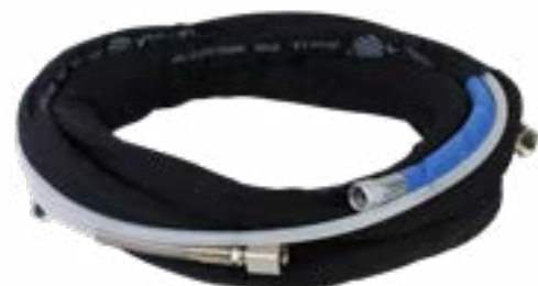
Air and product hose set for low pressure equipment. 8 x 15 mm. anti-static air hose and 6 x 8 mm. product hose with Nylon cover. Light and resistant hose. (see page 159)
